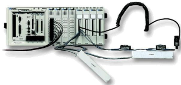
**Figure 10. Rack-Mount PC-Based Industrial Data Logging System**
